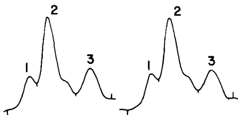
Figure 4. Scans of chromatograms of duplicate 5 \mu l blood serum samples; peak 1 is cholesterol, 2 is triolein, and 3 is cholesteryl oleate.
